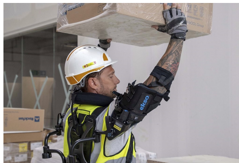
Construction worker wearing an exo-skeleton suit by Ekso Bionics
